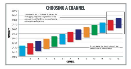
As evident in the picture above, the Wi-Fi channels are very wide, and have a lot of overlap. For this reason, most Wi-Fi users are placing all their traffic on channel 1, 6 and 11. These are the only non-overlapping channels available (except for some countries where there are two additional channels).
