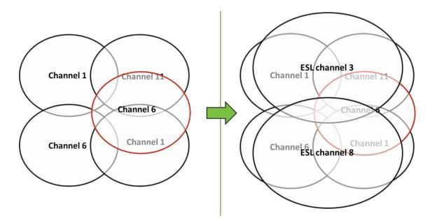
The picture above (left hand part) illustrates a typical Wi-Fi installation on channel 1, 6 and 11, where the red radio cell has been added to cover an area of weak radio coverage (for example due to high gondolas with liquids).
