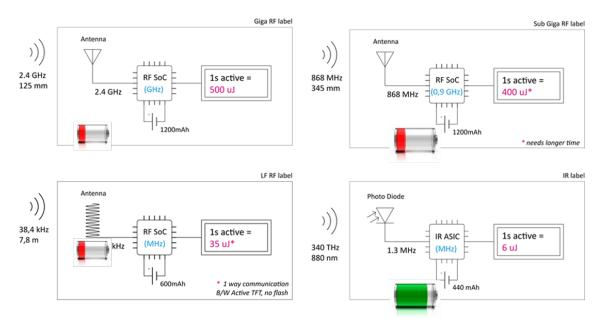
The battery cost of a listening event for a 2.4 GHz system is 83 times higher than an optical system (500  $\mu$ J versus 6  $\mu$ J). Because there is a limited availability of battery capacity, it leads to the following technical relationship between battery life and responsiveness:
